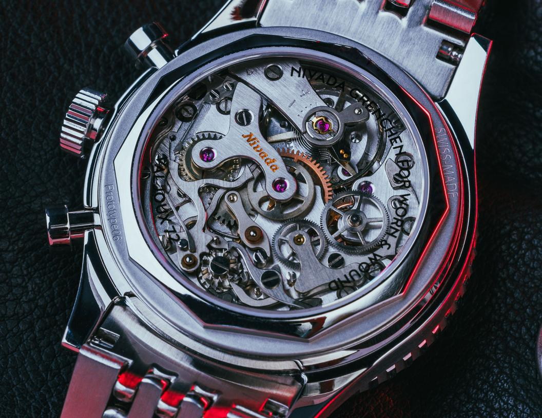
Made from 1918 to 1974, the Valjoux 72 powered various Rolex Daytona references, the Heuer Carrera 2447, the Nivada Grenchen Chronoking, and more. A column wheel chronograph with a frequency of 18,000 bph, the Valjoux 72 features a lateral clutch, and a balanced three-register design featuring running seconds, elapsed minutes, and hours, as well as an asymmetric pusher layout.
