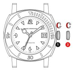
Position turn the crown unclockwise , unscrew crown To (2) position
