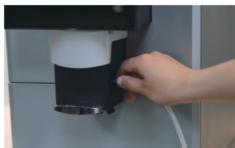
1. Connect milk pipe to machine
