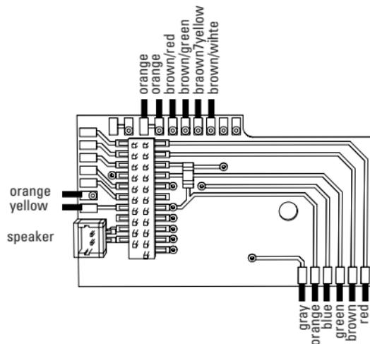
If the lighting is grounded to the locomotive or powered rail car's frame, this may cause flickering. If you don't want this, then the lighting must be insulated. We recommend replacing the light bulb(s) with the 604180 plug-in socket(s) and the 610080 light bulb(s). The ground is then connected to the orange wire.
