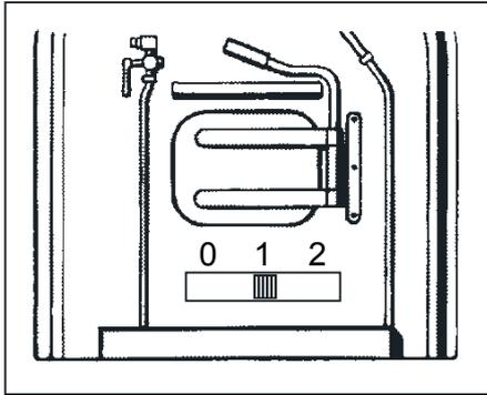
Fig. 1, Power control switch
