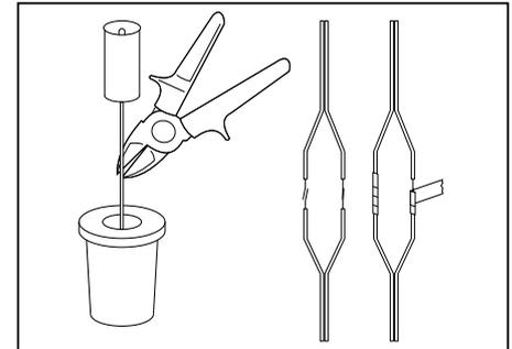
Fig. 3 & 4, Replacing the smoke unit
