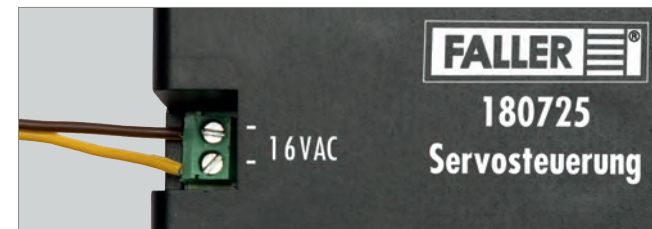
Fig. 2: Connecting the supply voltage
