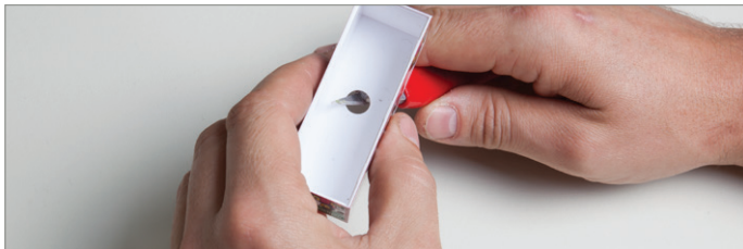
Fig. 38: Retouching the bore through the vehicle body
