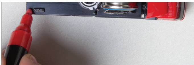
Fig. 13: Mark the polarity of the charging socket, vehicle body inside
