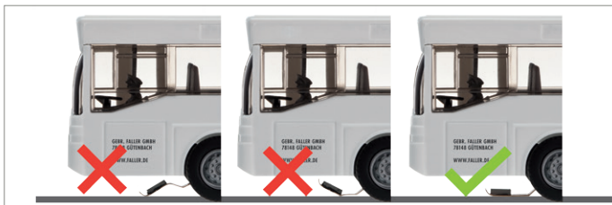
Fig. 51: Adjusting the steering rod
