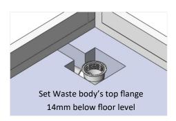
3. Measure and set up the position for the Athena Easyclean waste body. PLEASE NOTE: when setting the waste position set the top flange 14mm below the level of the floor as the shower tray's waste area has a spigot protruding down from its underside. It is also recommended that the waste connection be water tested. Sweep the area to remove any debris.
