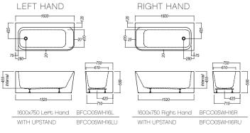
250 litre water capacity 250 litre water capacity Water capacity measured 80mm from top edge of bath
