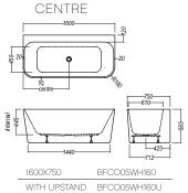
WITH UPSTAND BFC005WH180U 240 litre water capacity 295 litre water capacity 42 Dimensions are nominal
