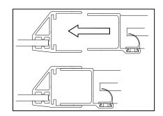
Using the clear adhesive tapes provided hold the door assembly to the Take up Panel
