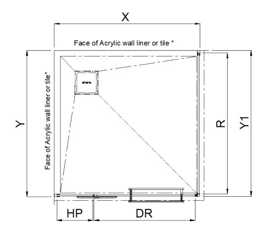
Note: \* Maximum permissible Tile Thickness when Installing on Athena SlateForma Shower Tray = 10mm
