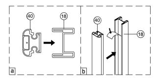
Clean the glass edge by No.26. Remove the double-side tap a little bit and stick the joint to the glass edge,doing them on the same time.
