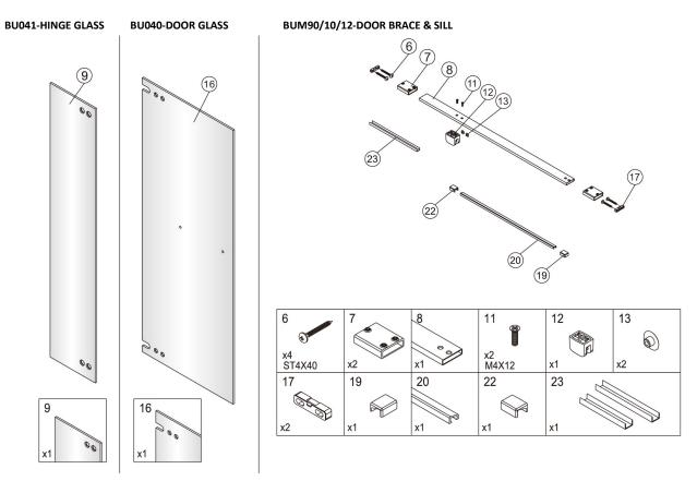
N:B - For 1000mm & 1200mm Door sets there are two of Item 23 supplied, the shorter of the profiles is used **only on Alcove Tile Door Sets** while the longer profile is used on all other Door sets.
