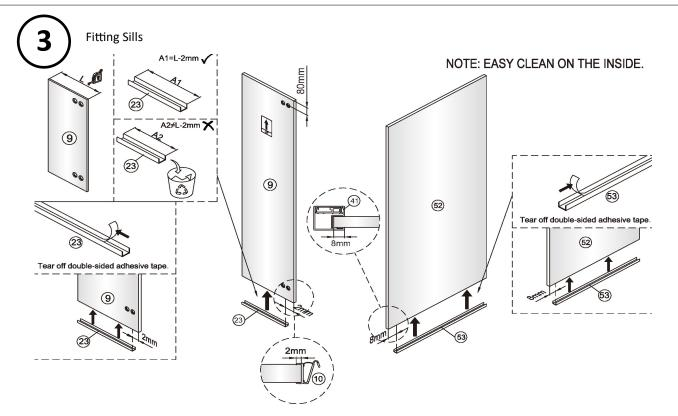
N:B - For 1000mm & 1200mm Door sets there are two of Item 23 supplied, the shorter of the profiles is used **only on Alcove Tile Door Sets** while the longer profile is used on all other Door sets.
