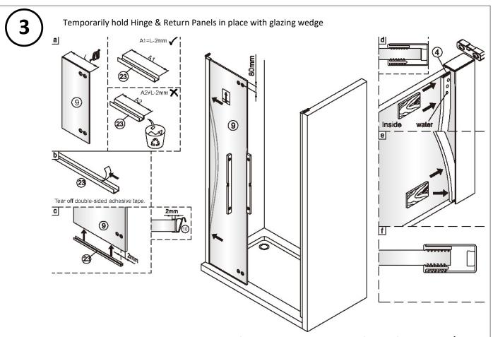
N:B - For 1000mm & 1200mm Door sets there are two of Item 23 supplied, the shorter of the profiles is used **only on Alcove Tile Door Sets** while the longer profile is used on all other Door sets.
