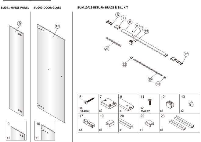
N:B - There are two of Item 23 supplied, the shorter of the profiles is used on the Alcove Tile Door Sets, all other Doors use the longer profile
