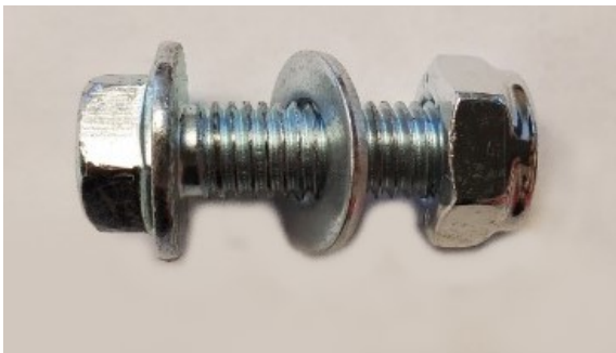
Figure 6: Flanged bolt, washer, and lock-nut diagram. 14mm head, 17mm flat-washer, and 17mm lock-nut. Flat-washer will be on the lock-nut end of the bolt when installed.
