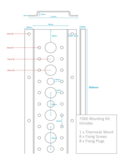
Designed for multiple rail installation of our Single Bar 12V Towel Rails.
