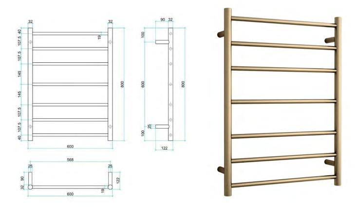
This rail has Multiflex wiring which means that there is a connection point on both the left and right hand side of the rail and the lead can be connected to either side. Being a dry element rail, this can be mounted either way up meaning the wiring can be from any of the four mounting points.
