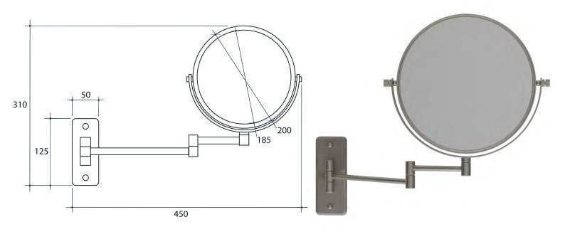
Maximum Distance From Wall 330mm Length From Wall When Folded - 30mm
