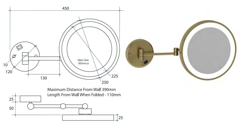
Note: All dimensions are in millimetres (mm)
