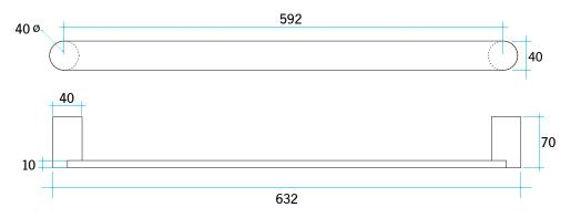
Note: All dimensions are in millimetres (mm)
