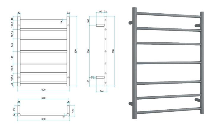
This rail has Multiflex wiring which means that there is a connection point on both the left and right hand side of the rail and the lead can be connected to either side. Being a dry electric element rail, this can be mounted either way up meaning the wiring can be from any of the four mounting points.
