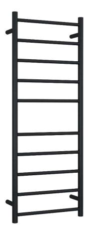
This rail has Multiflex wiring which means that there is a connection point on both the left and right hand side of the rail and the lead can be connected to either side. Being a dry electric element rail, this can be mounted either way up meaning the wiring can be from any of the four mounting points.
