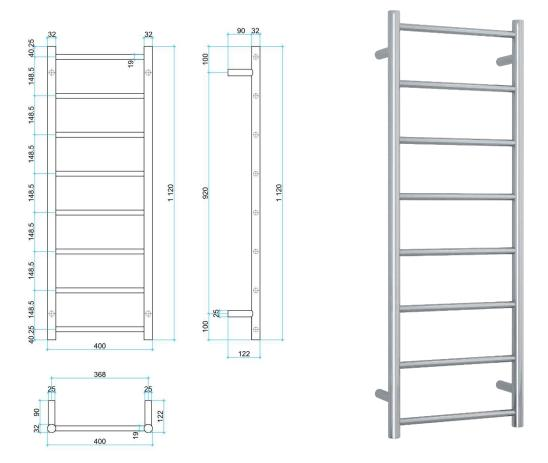
This rail has Multiflex wiring which means that there is a connection point on both the left and right hand side of the rail and the lead can be connected to either side. Being a dry electric element rail, this can be mounted either way up meaning the wiring can be from any of the four mounting points.
