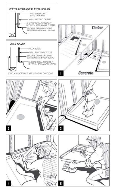
www.polymore.com.au sales@polymore.com.au Water resistant plaster board installation. Glasstone shower base has a tile flange. Place base against framework, install water resistant plaster board directly on top of tile flange and seal joint with flexible silicone sealant.
