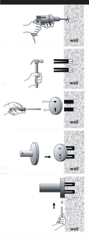
1. Put the fixing blocks (piece) over on the right place on the wall , and stay level, use marking pen through the holes of fixing block to mark out fixing spots on the wall. Then drill holes by electric hand drill with 6mm drilling bit on the spots.
