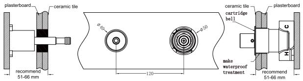
6.Put cartridge bell onto body and do waterproof treatment.
