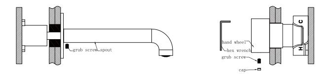
7.Put plate, washer and spout onto body successively, tighten grub screw of spout firmly by hex wrench.
