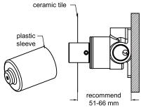
2.Connect cold water hose and hot water hose take off plastic sleeve and conduct water pressure test for leak.
