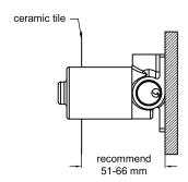
1.Fix body on noggin and ensure installation depth is 51-66mm from noggin to ceramic tile.
