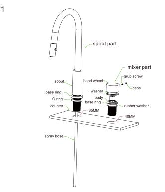
1.Drill a 35mm (for spout) and a 40mm (for mixer) through-hole on the counter. (The counter thickness must between 20mm to 40mm)
