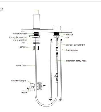
Slide rubber washer, triangle plate and steel washer and lock nut onto spout part in a row according above diagram. Then slide rubber washer and nut onto mixer part .
