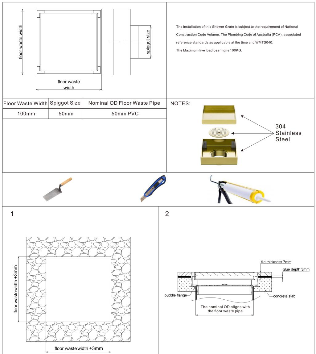
1. Cut grate to suit floor waste allowing at least 3mm of clearance in overall length to facilitate removal for cleaning.
