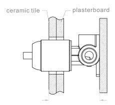
4. Remove the plastic sleeve of body.
