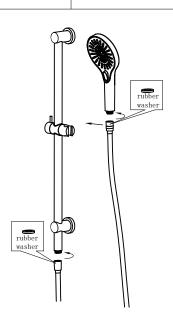
5. Connect shower rail and hand shower with hose. TEST & CHECK FOR LEAKS.
