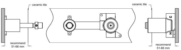
1. Fix body on noggin and ensure installation depth is 51-66mm from noggin to ceramic tile.
