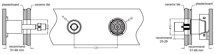
3.Adjust connecting rod and ensure depth is 25-28mm from the front of adaptor to ceramic tile.
