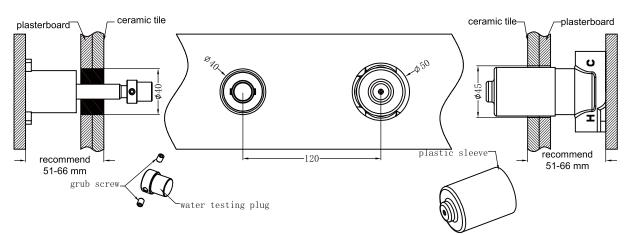
5. Remove plastic sleeve, grub screw and water testing plug.
