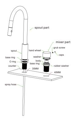
1.Drill a 35mm (for spout) and a 40mm (for mixer) through-hole on the counter. (The counter thickness must between 20mm to 40mm)
