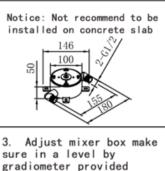
1. Mixer box should not finish more than 2mm above finish tile level \$\phi\$125 (4-\$\phi\$8D≥65)
