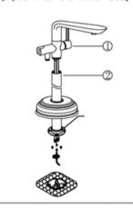
8. Fit floor cover plate onto the extension tube
