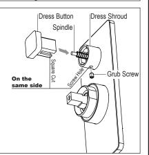
5 Push on Mixer Handle Fasten Grub Screw to secure Mixer Handle.
