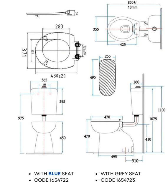
SUITE INCLUDES: CHROME RAISED BUTTON, VC CISTERN, STAINLESS STEEL FLUSHPIPE, SKIRTED PAN, SINGLE FLAP SEAT
