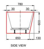
WHERE BATH CONNECTS TO A WALL, IT MAY HAVE A 5MM VARIATION THAT WILL REQUIRE CAULKING FOR FLUSH FINISH TO WALL - WALLS & FLOOR MUST BE STRAIGHT BEFORE INSTALLATION
