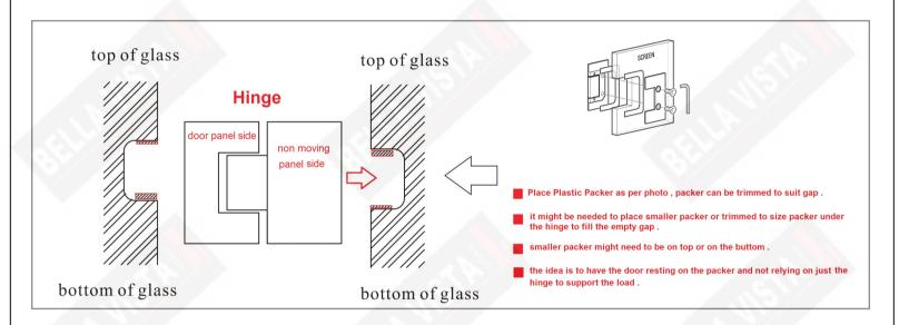
PUT THE SUITABLE SIZE PACKER BETWEEN HINGE AND GLASS AS PER PHOTO TOP OR BOTTOM TO STOP THE GLASS FROM DROPPING. PACKERS CAN BE TRIMMED TO SIZE IF NEEDED TO FIT BETWEEN GLASS AND HINGE BODY
