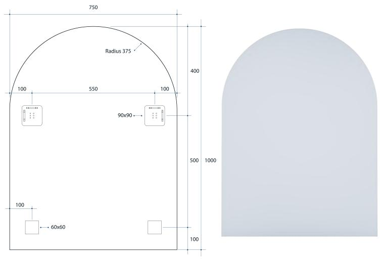
Note: All dimensions are in millimetres (mm)
