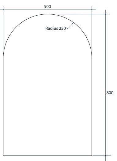
Note: All dimensions are in millimetres (mm)
