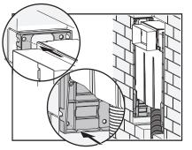
7. Secure the flush pipe to the masonry utilising 2 of the screw holes in the flush pipe mounting box and slide blue flush pipe tiling box over flush pipe.
