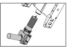
5. Lubricate 'O'Ring on cistern tail using soapy water and slide flush pipe on.
