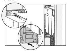
**5.** Secure the flush pipe to the Nogging utilising 2 of the screw holes in the flush pipe mounting box and slide blue flush pipe tiling box over flush pipe.
