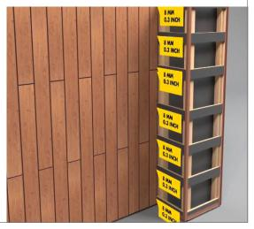
• Fix the cladding with SFS Intec HPL Fast Fixing Screws.
