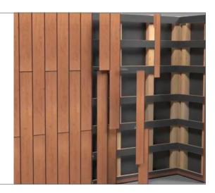
• For the corners, cut a cladding plank to size.
