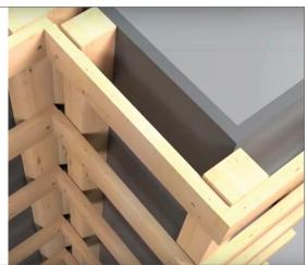
• Attach strips of **EPDM Rubber Gasket** at least as wide as the horizontal batten.
