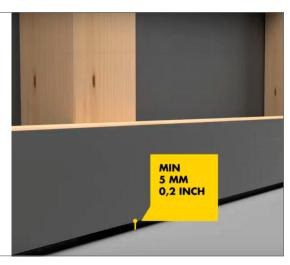
• Ensure there is sufficient space behind the vertical battens for natural ventilation.
