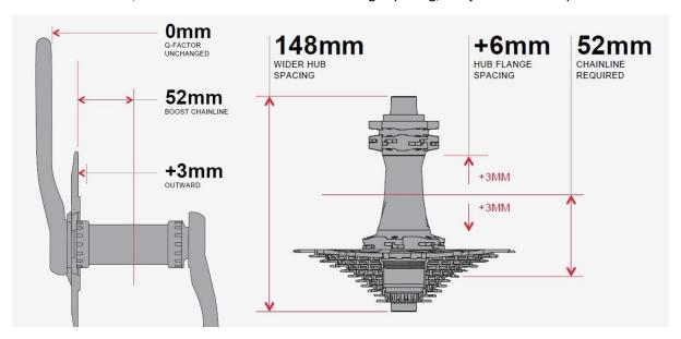
**BOOST 110** uses a 15mm thru axle and moves hub flanges outboard by 5mm when compared to 100mm hub standards. This 5mm outboard movement affects the spoke bracing in the same way as the 3mm shift on 148mm rear hubs, increasing spoke angles and creating, "the stiffness of a 26-inch wheel" in the front as well.
