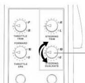
当您旋转方向轮时,调节转向比率可以帮助您改变车轮转向幅度。 Adjust the steering rate can help you to change the wheel steering range.
