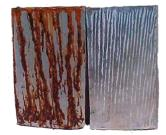
Salt Spray Test: Coated panels were exposed for 14 days to salt spray per ASTM- 117 test procedure at an independent testing lab. The results conclusively indicate that metal surfaces protected using Flexi-Film® provide superior resistance to environmental elements.
