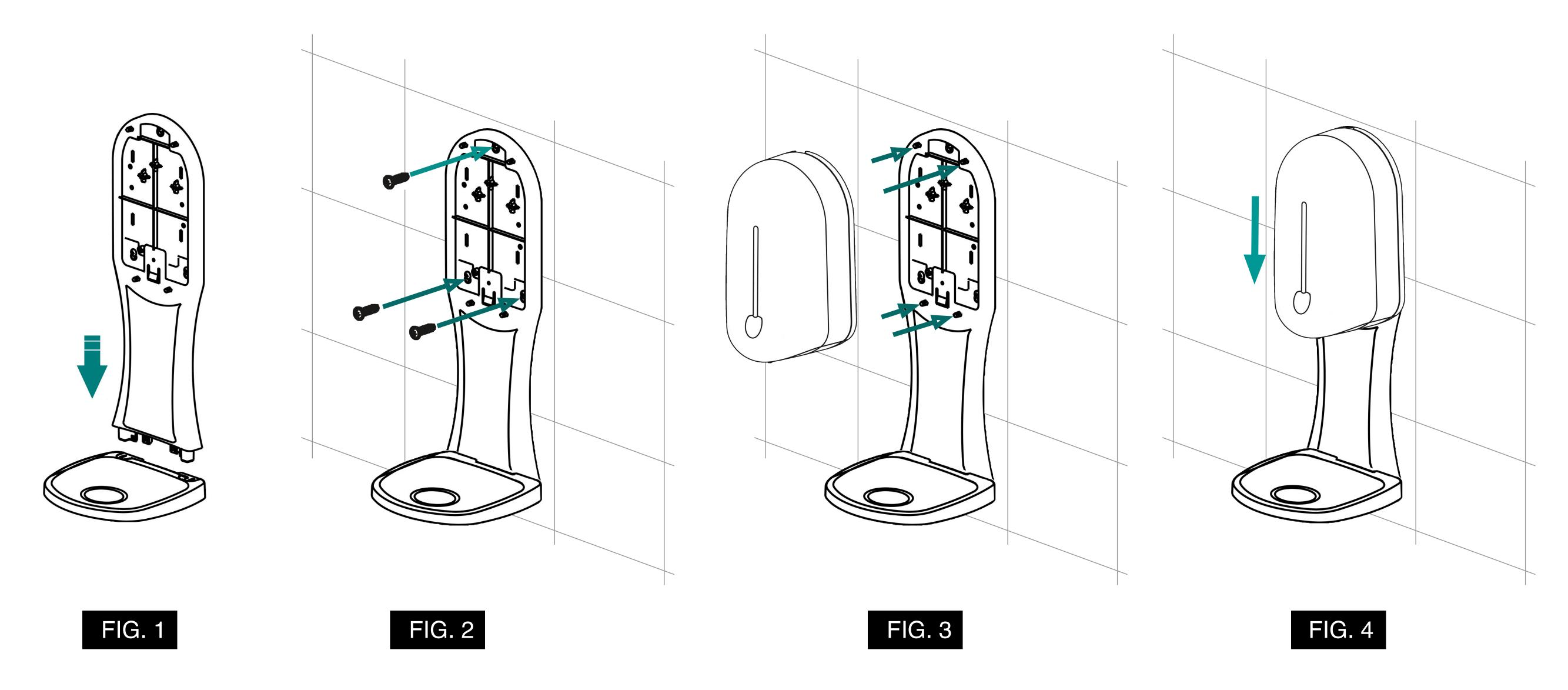
**Step 3** Align the 4 holes in the back of dispenser with the 4 hooks on the backsplash guard. Push the unit against the backsplash guard (FIG. 3) and then push the unit down towards the drip tray until the top of the unit is flush with the top of backsplash guard (FIG. 4).
