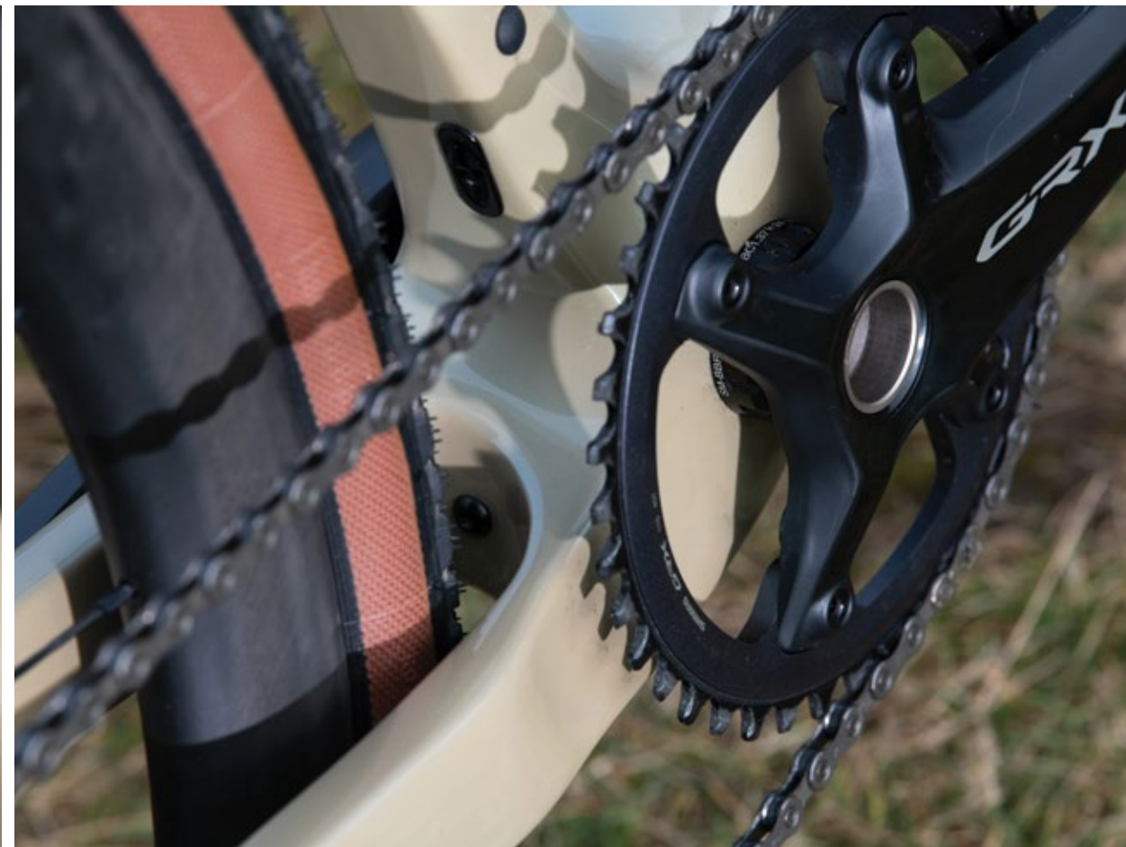
The On And On has a lot of bottom bracket drop – how far the bottom bracket sits below the wheel axles – which lowers the rider's centre of gravity for extra stability
