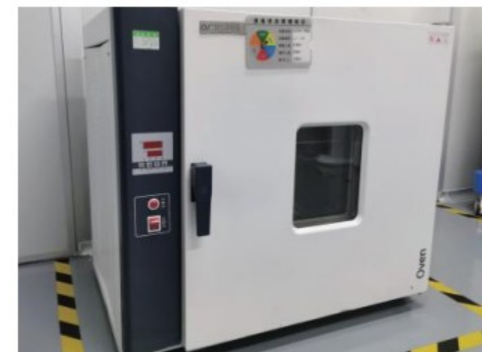
Electric heating blast drying oven
