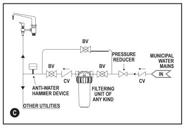
CV = Check Valve, BV = Ball Valve
