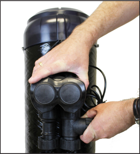
Attach water meter, spacer and bypass assembly. Lubricate connector O-rings with a food grade silicone before installing on bypass. HAND TIGHTEN ONLY!
