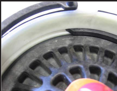
Install the angled lead tip of the retaining ring into the groove.
