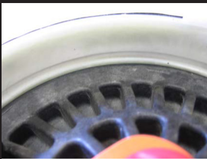
Ensure the top Pressure Release Cap Lid is installed to fully expose the retaining groove.
