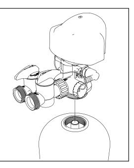
After media is added, remove the plug from the distributor tube, and fill the tank the rest of the way (up to the bottom of the tank threads) with water. This will allow the filter media to soak while the installation process is completed. Make sure that tank threads are clean and free of any media fines, and screw the control valve back onto the tank.
