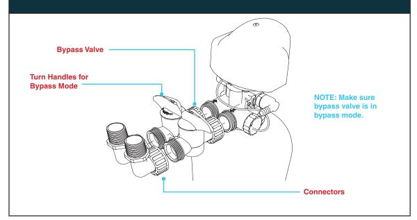
Turn off main water supply and open nearest cold faucet to relieve pressure. Cut water supply line, and connect plumbing to the inlet and outlet accordingly. Note: Inlet and outlet connections are 1" NPT. Additional piping and / or fittings may be necessary
