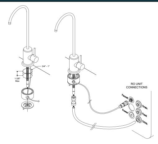
**Faucet Installation -** Drill a 3/4" hole for the stainless steel faucet and install, being sure that the faucet cable exits through the gap in the supplied spacer without being pinched.. Connect faucet cable to the FAUCET port on the RO System.
