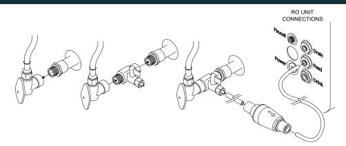
**Inlet Water Port** - Cut a short segment from the supplied 1/4" tubing (~12") to install between the shutoff valve and the pressure reducer. The remaining tubing is installed between the pressure reducer and the RO System's 'FEED' port. Also, the pressure reducer needs to be installed with the arrow on the reducer pointing in the direction of flow from the water supply to the RO unit.
