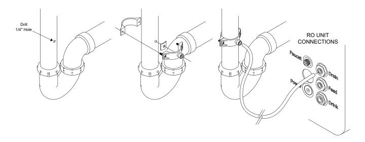
**Drain Water Port -** Drill a 1/4" hole in the existing drain well above the trap. Remove the center punch-out from the included saddle clamp gasket and adhere the gasket over the 1/4" hole in the drain pipe. Install the drain saddle clamp with the port centered over the hole in the drain pipe.
